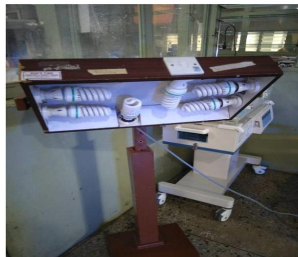
**Figure 1: Locally-fabricated CFL bulb phototherapy device (AVA-2014)**
